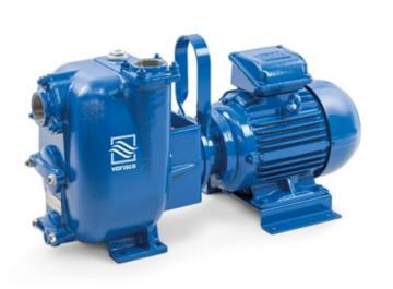
**Product Data** Suction port Threaded - 3" ISO 228 (BSP) Delivery port Threaded - 3" ISO 228 (BSP) Qmax 105 m<sup>3</sup>/h - 1750 l/min (462 USgpm) Hmax 23 m (75 ft) Solids handling 40 mm (1,5 ") Motor power 7,5 kW - 10 HP Motor type **IEC** standard Winding for inverters **Cast iron frame** Motor brand WEG W22 Premium Weight 144 ka
